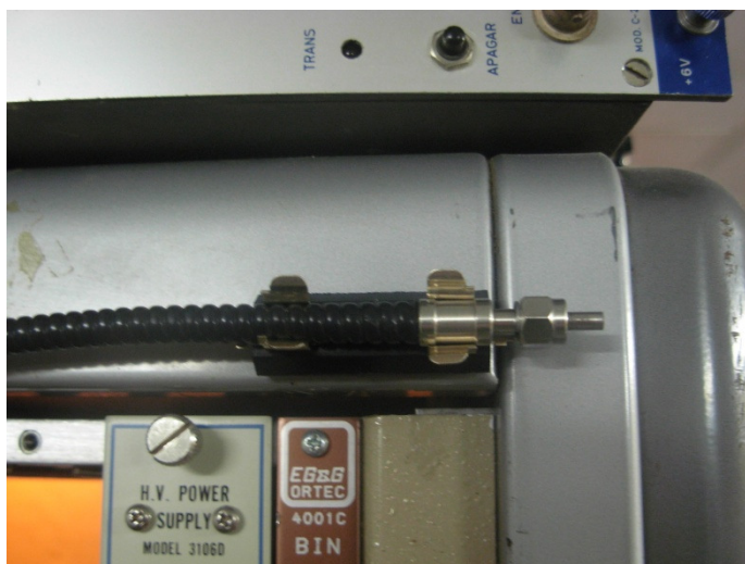
Figure 10 – Photography of the optical fiber in the test position to calibrate the system and monitor its sensitivity; also in the picture is the beam current meter.
