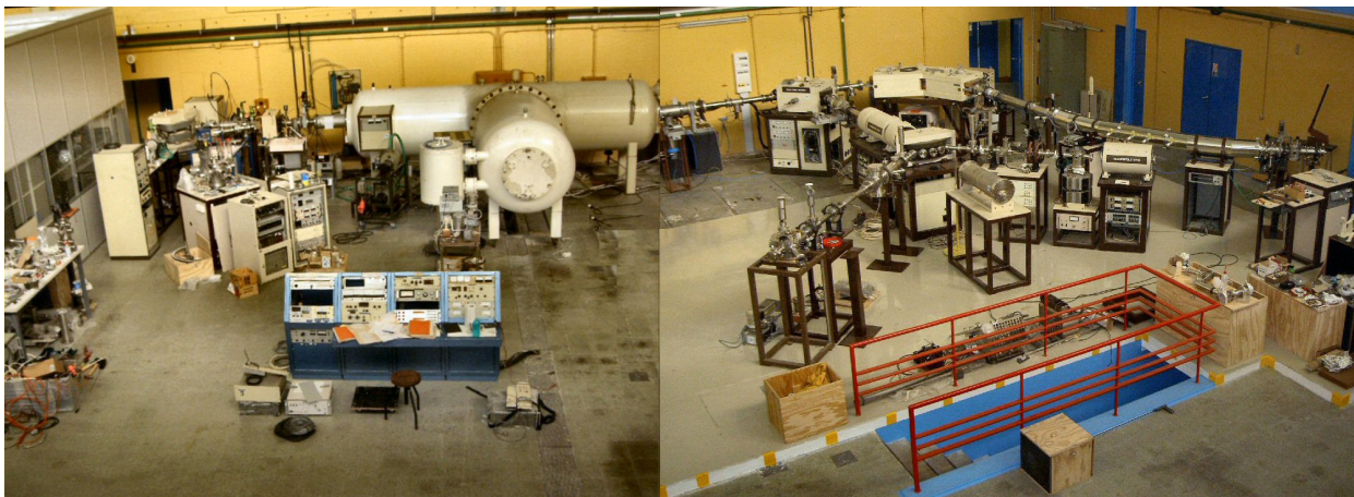
General view of the 3 MV Tandem accelerator equipped with an accelerator mass spectroscopy (AMS) system with a lateral resolution of 30 \mu\text{m} .
