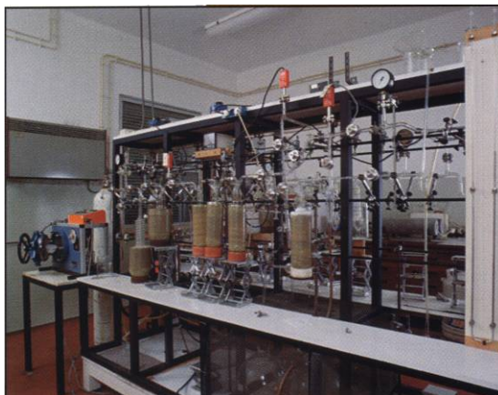
Benzene synthesis line of the radiocarbon dating unit.
