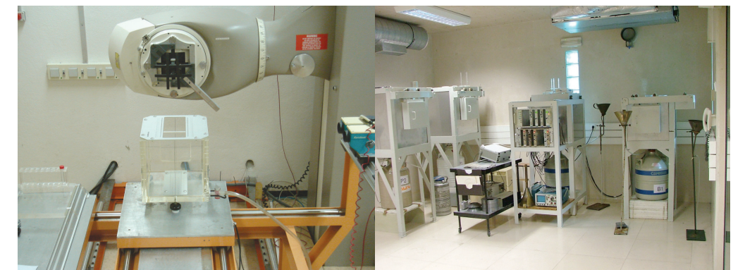
UPSR Infrastructures: Cobalt-60 irradiator (left) and HPGe detectors for gamma spectrometry (right).
