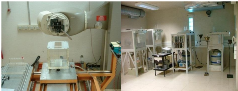
UPSR Infrastructures: Cobalt-60 irradiator (left) and HPGe detectors for gamma spectrometry (right).
