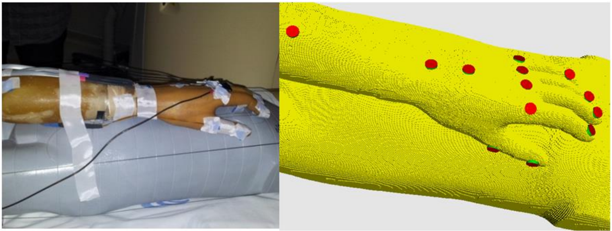
Fig. 2: Dosimetry of the medical applications of ionizing radiation: CT-fluoroscopy: hand phantom (left) and model (right, the red dots correspond to dosimeters).
