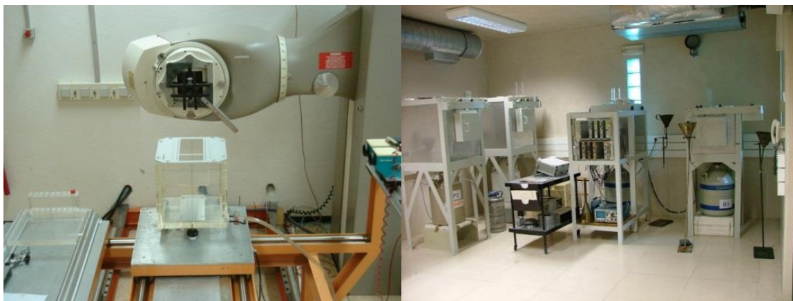
Fig. 5: Infrastructures at the UPSR: Cobalt-60 irradiator (left) and HPGe detectors for gamma spectrometry (right).
