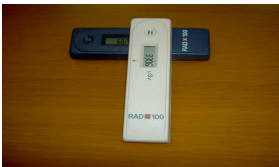
Fig. 17: RAD X100: light weight personal radiation dosimeter.
