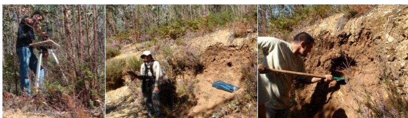
Fig. 3: Soil sampling and field gamma spectrometry in Central Portugal.
