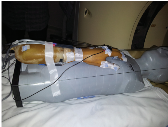
Dosimetry of the medical applications of ionizing radiation. Exposure of the extremities of the medical doctors in CT-fluoroscopy: physical hand phantom with dosemeters (left) and implemented computational model (right, voxel phantom with the red dots corresponding to dosemeters).
