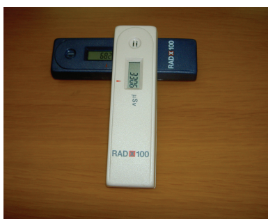
RADX 100: light weight personal radiation dosimeter.
