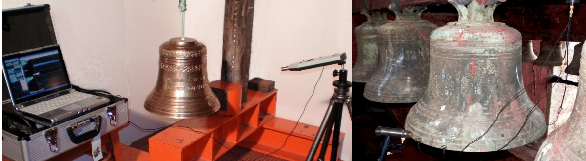
Fig. 1 - Experimental identification of bell modes : laboratory bell (left), Maфра carillon (right).
