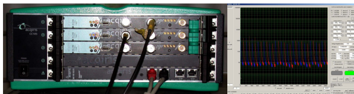
Legend: LEFT DIGIPAC main core, consisting of 3 dual cards integrating each one, two digitizer Aquiris and two FPGAs for digitalizing data and processing RIGHT data acquisition of 30 time spectra / combinations for each pair of detectors in coincidences \gamma_1 - \gamma_2 , produced during the ^{61}\text{Cu}/^{61}\text{Ni} PAC experiment.
