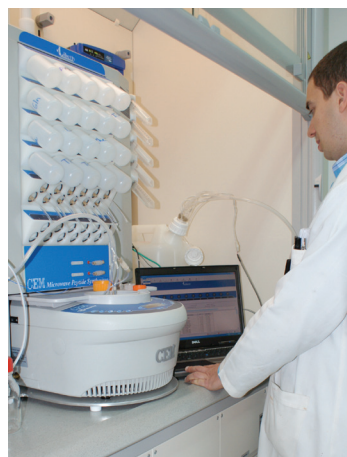
(Left) Automated Microwave Peptide Synthesizer.
