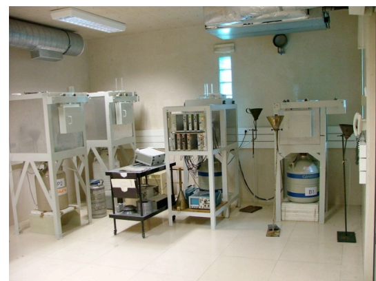
HPGe detectors in the gamma spectrometry counting room.
