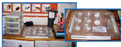
Fig. 2. Placement of the passive filters in the classrooms.
