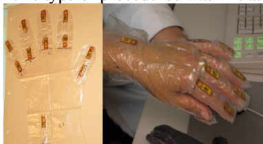
Fig.1 Glove with extremity dosimeters for dose mapping of the hand.
