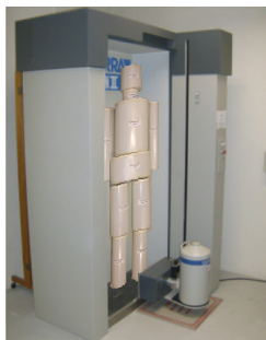
Fig.2 WBC and the BOMAB phantom
