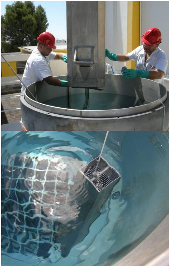
Fig 1. Loading into the TN-MTR transport cask of an irradiated (top) and a fresh fuel assembly (bottom).
