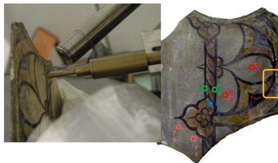
Fig.: Experimental mount and glass fragment sample analysed in the external beam. Coloured dots indicate analysed spots.
