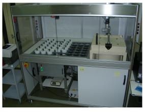
Samples can be positioned at different distances from the germanium detector by placing rings. Gamma spectra in digital form enter the k<sub>0</sub> IAEA program for direct calculation of the concentrations. A Partisol Plus sequence air sampler was also acquired to collect
