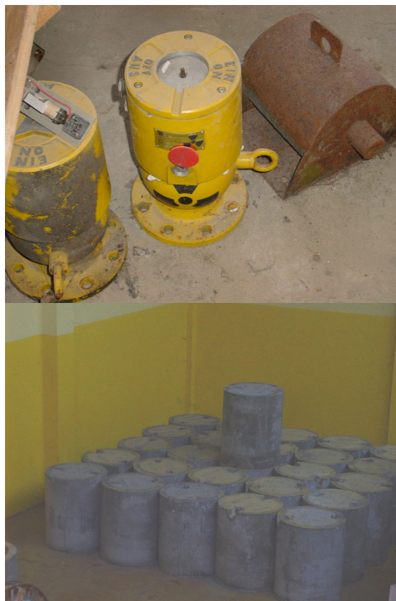
Figure 1 – Examples of sealed sources conditioning within concrete drums to be disposed in a near surface repository.
