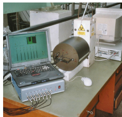
Fig. 3. The Monoblock neutron spectrometer with an evaluation computer.
