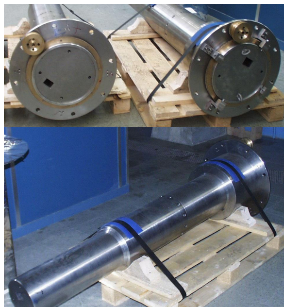
Fig. 2. Pictures of the in-pile collimators. Top -view of the outer carter and rotor flanges; bottom – rear view of one of the in-pile collimators.
