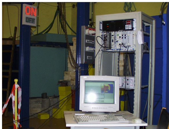
Fig.1. EPA - View of the EPA Spectrometer data acquisition and command and control electronics
