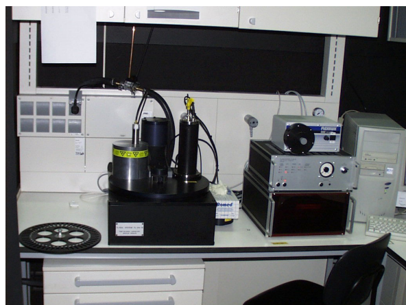
Fig. 1. Risoe D-15 Luminescence Reader of the luminescence laboratory.
