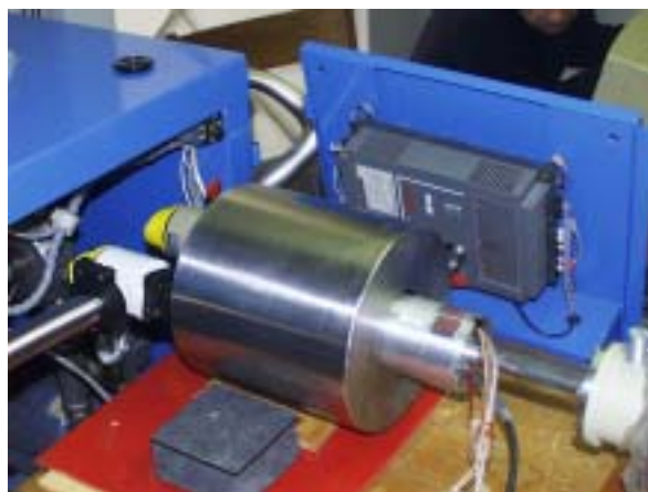
Fig. 1: View of the Marinelli beaker with a HPGE detector installed at the AIRMON-91 system during calibration measurements.
