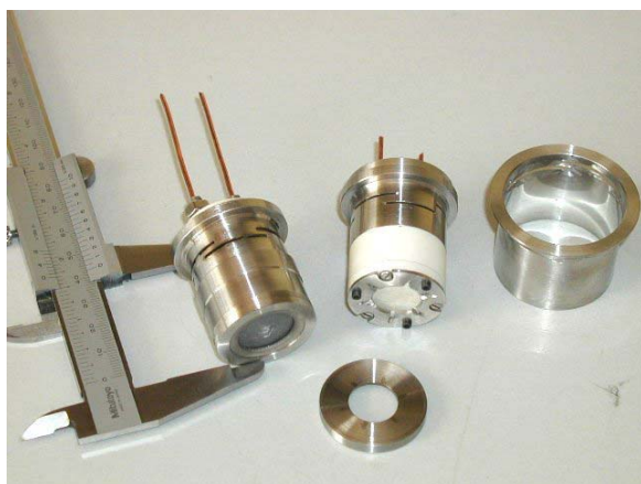
New substrate holders, which can be heated up to 800°C.
