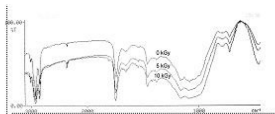
Fig. 2 - FTIR spectrum of the solid phase of an Agro-industry before irradiation (0 kGy) and after \gamma irradiation (5 and 10 kGy).
