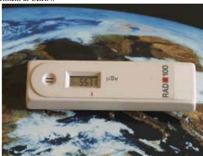
Figure: Lightweight personal Radiation Dosemeter, made in ITN
