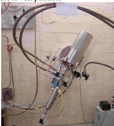
Fig. 1: The ITN Pulse Tube in the worst position (150°)!
