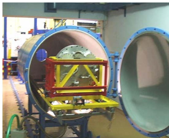
Fig.3 EPA - detector housing and PSD detector on its platform
