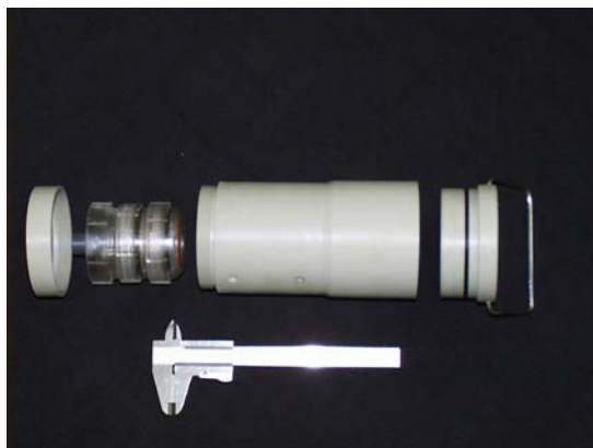
Fig.2 View of the URSA and PM10 separator.
