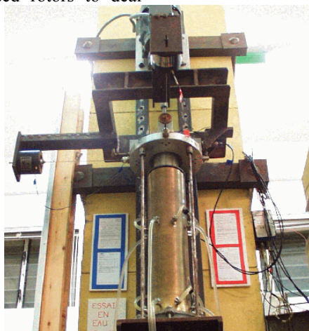
Experimental set-up for rotor-flow interaction tests.
