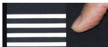
Figure 2. Picture of the thin ribbon developed. Each element is 3.5 mm wide and 0.2 mm thick.
