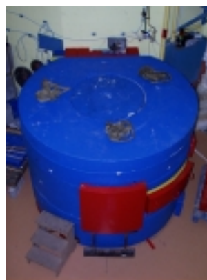
View of the shielding that surrounds the monochromator of the two – axis diffractometer, DIDE.
