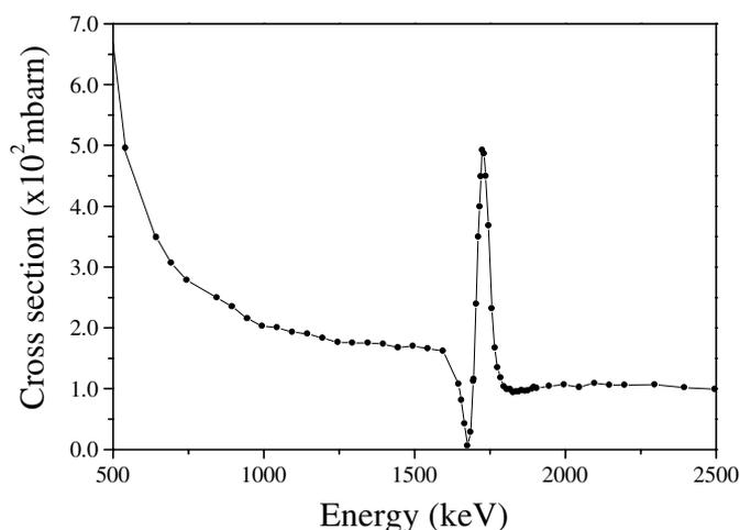
Fig. 1 Measured cross section for the reaction  $^{12}\text{C}(p,p)^{12}\text{C}$  for the 140 scattering angle.
