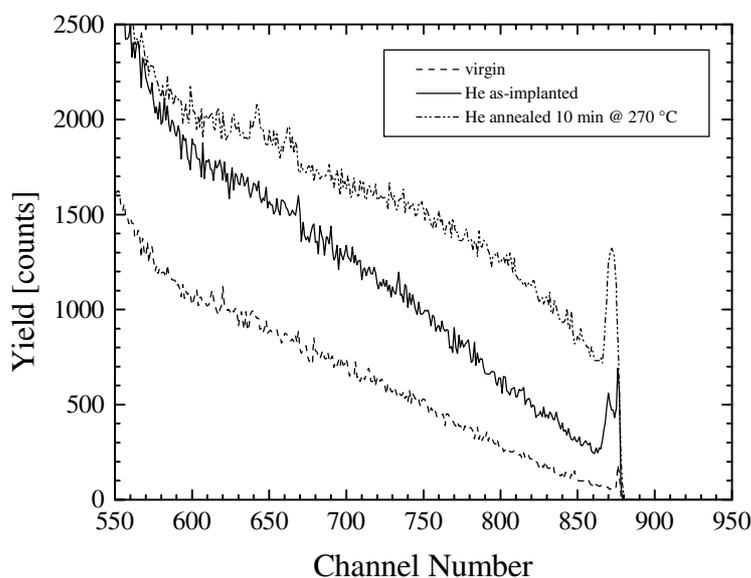
Fig. 1: RBS/channeling spectra of virgin, as-implanted and heat-treated LiNbO<sub>3</sub> for 4 MeV He<sup>++</sup>
