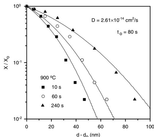
Fig. 1: Fit of Ir depth profiles of samples annealed at 900°C for different anneal times.
