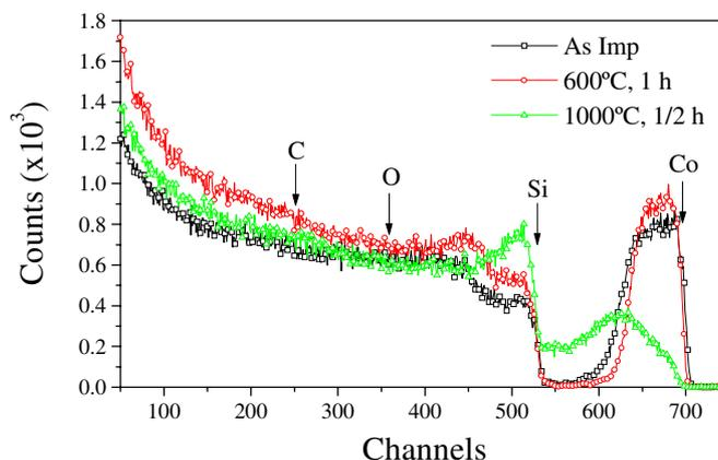
Fig. 1 RBS results of a porous Si sample implanted with  $2 \times 10^{17}$  at/cm<sup>2</sup> Co at 350°C and annealed at different temperatures (600°C e 1000°C).
