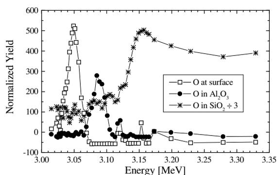
Fig. 1: Energy dependence of the resonant scattering yield for the three oxidized regions
