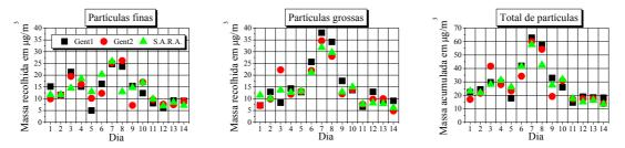
Fig. 1 – Gravimetric mesurement of collected masses by the three samplers, S.A.R.A. being the automatic filter change system and the others two identical Gent PM10 samplers. Data are shown for fine particles (partículas finas), coarse particles (partículas grossas) and the sum of both (Total de partículas).
