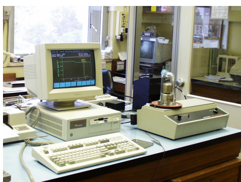
Fig.1: Thermal analysis equipment. (DSC module and PC controller).
