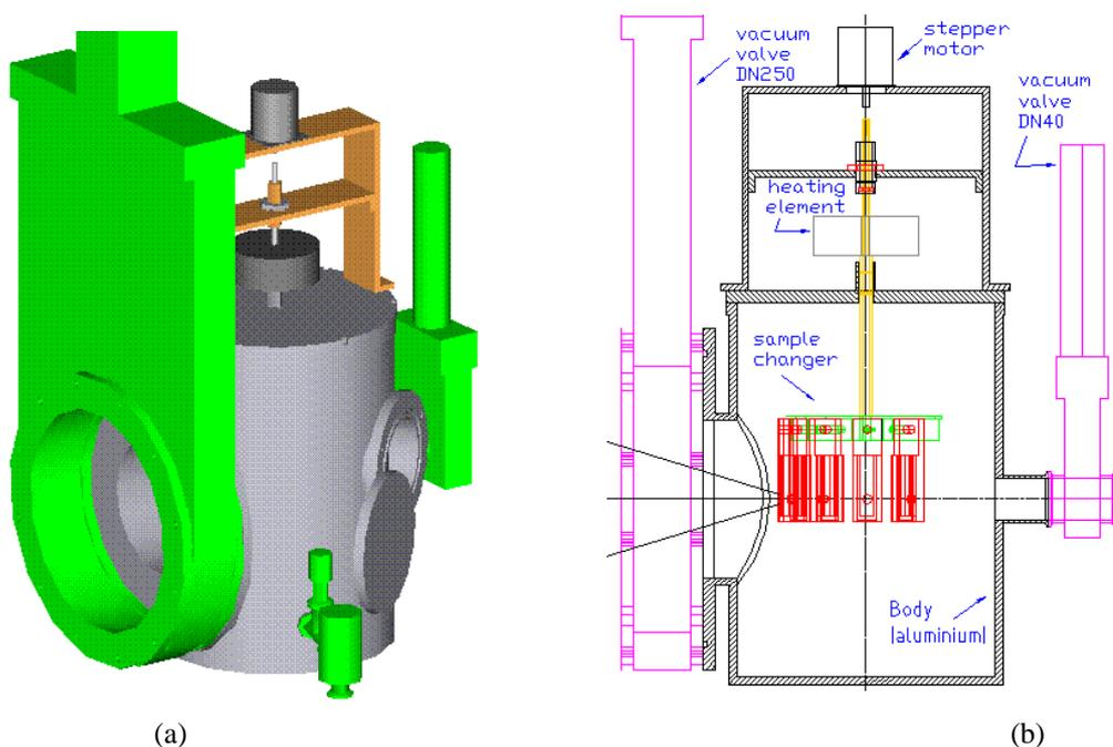
Fig.1 Sample Chamber (a) 3-D general view (b) cross-section view
